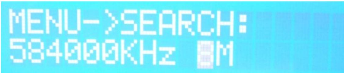
Diagram 6: When the frequency setting is complete, the channel bandwidth selection and transmitter of the same value, and press "OK" button to search
